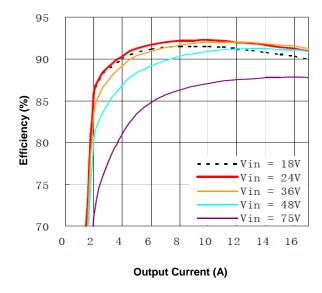
Figure 1. Efficiency vs. Load Current
