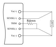
Figure 17. Circuit to Decrease Output Voltage
