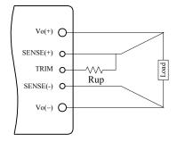
Figure 18. Circuit to Increase Output Voltage
