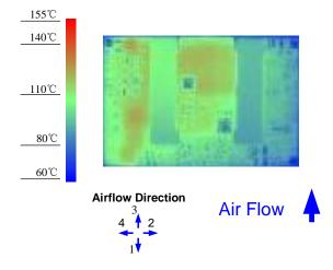
Figure 12. Thermal Image for Airflow Direction 3 (13.8A output, 55°C ambient, 200 LFM, typical Vin, open frame unit using soldering interface)
