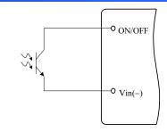
Figure 14. Opto Coupler Enable Circuit
