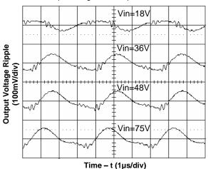
Figure 5. Output Ripple Voltage at Full Load
