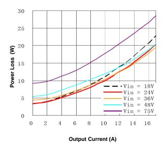
Figure 2. Power Loss vs. Load Current
