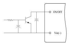
Figure 15. Open Collector Enable Circuit
