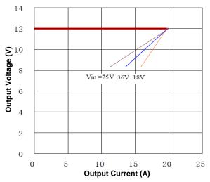
Figure 10. Output Characteristics
