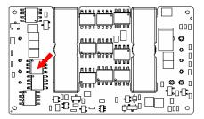
Figure 19. Temperature Monitoring Location
