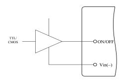
Figure 16. Direct Logic Drive
