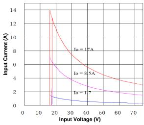
Figure 9. Input Characteristics
