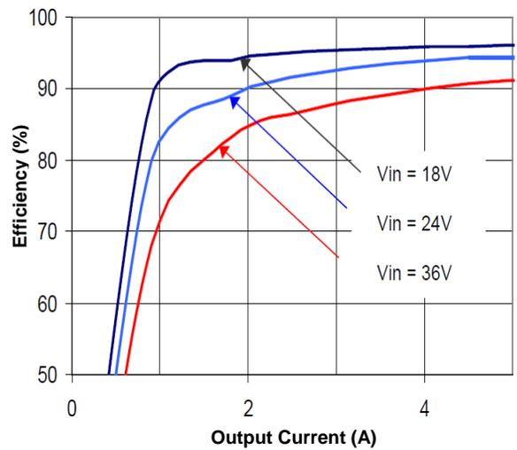
Figure 1(b). Efficiency vs. Load Current (25°C, 12V)
