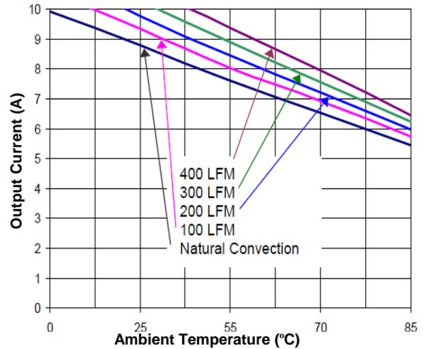
**Figure 11.** Current Derating Curve for 5V Output
