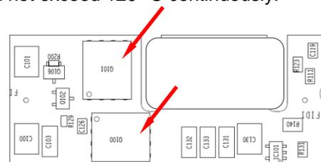
Figure 15. Temperature Monitoring Locations
