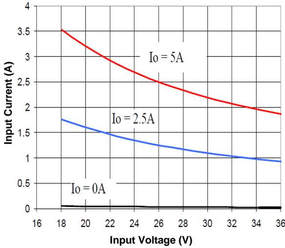
Figure 2. Input Characteristic (12V output)
