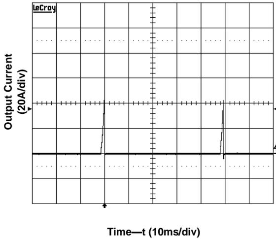
**Figure 10.** Short Circuit Current ( $V_{in} = 24V$ )
