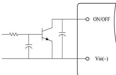
Figure 13. Circuit for Negative Logic Control
