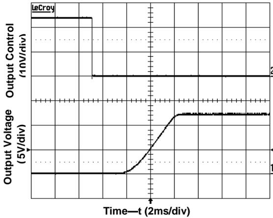
Figure 4. Start-Up from Enable Control
