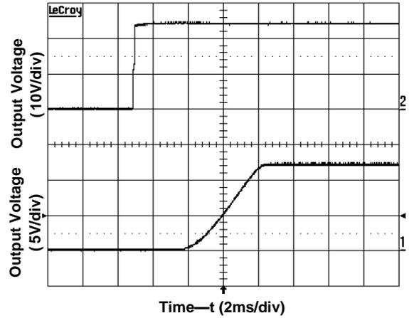
Figure 5. Start-Up from Application of Input Voltage
